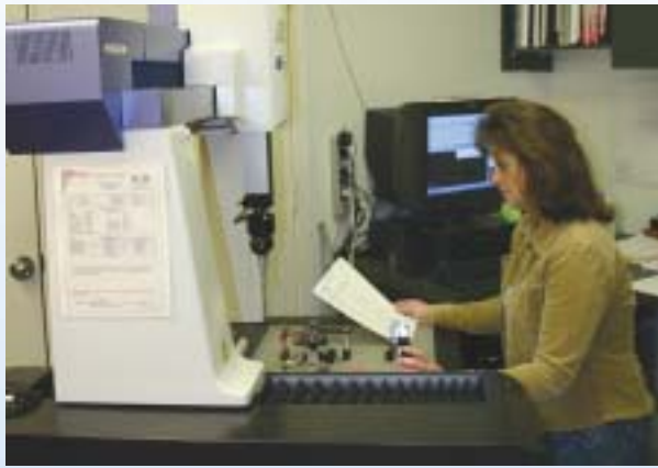
Quality assurance is a top priority at all Ashley Ward, Inc. facilities, which is why we utilize state-of-the-art measuring equipment like this Coordinate Measuring Machine (CMM).
